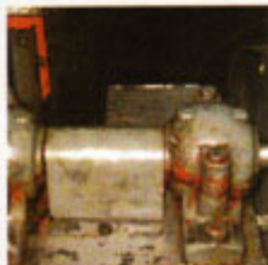
Mechanical: Overheating bearing at pulley end
