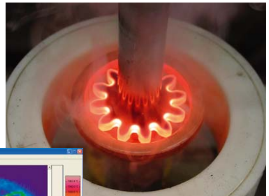
Laboratory arrangement at a customer of IMPAC systems. By analysing the temperature distribution the induction hardening process is optimised.
